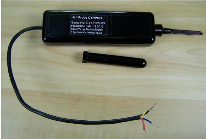
For measuring the magnetic field, please put the rear side of the Hall probe on the surface of the measured magnet or at the measuring point of a magnetic field carefully. The probe doesn't give any output signal if one places the front side to the surface of the measured magnet.
