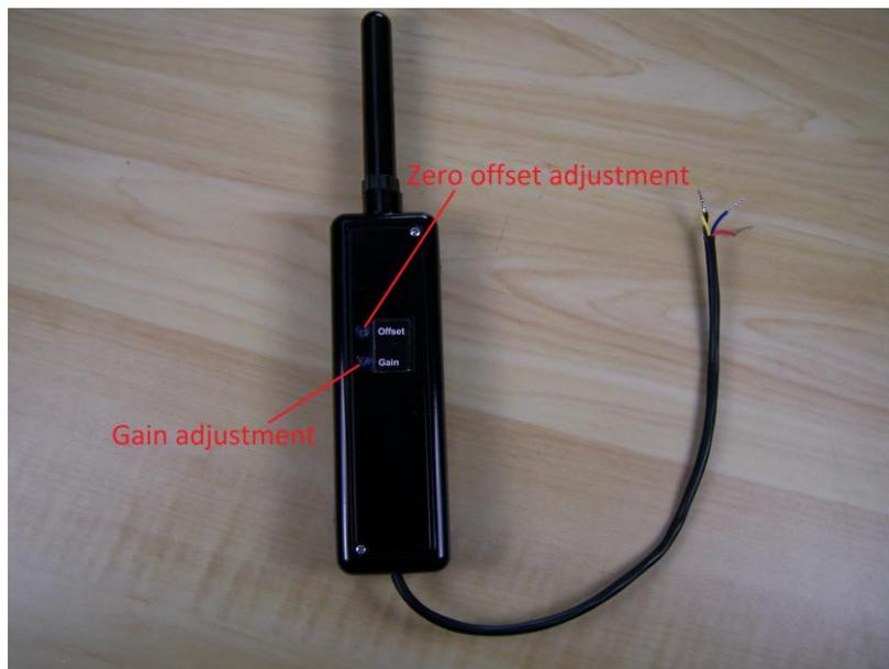
The zero offset can be adjusted by the potentiometer named with "Offset". It is recommended to set up a zero point at about 8mV, which means a zero point deviation of about 0.2%. By using this method, a dead zone, which causes decreasing sensitivity and nonlinear behavior, can be avoided effectively.
